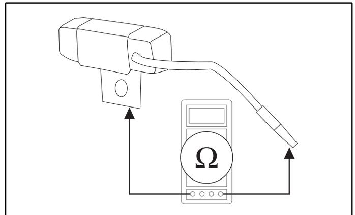
**Checking the electric starter**
