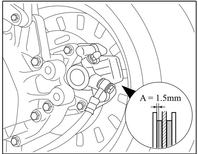
■ **Replacing the brake pads**
