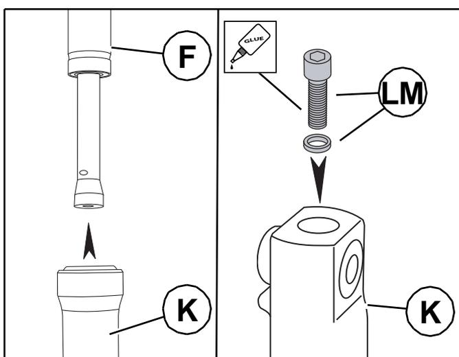
Install the stanchion assembly screw and its seal (LM).
