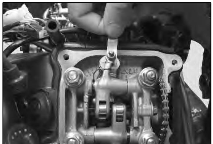
■ **Checking the valve clearance**
