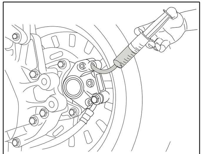
Draining the front brake circuit:
