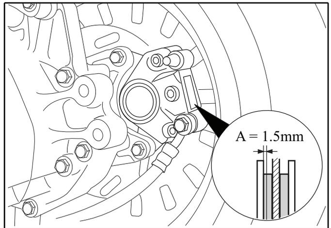
■ **Replacing the brake pads**
